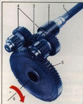
1 Side shaft, seated in two bearings, 2 Toothed segment joint, 3 Floating pinion shaft, 4 Twin layshaft, 5 Rear axle half-shaft, spur gear with twin drive, 6 Rear wheel
