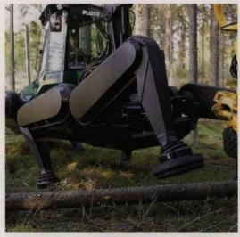
Timberjack's new machine concept has been developed to test the suitability of walking technology for mechanical hervesting. The prototype was introduced in 1995 and is not yet commercially available.
